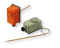
TC2 is a boxed immersion thermostat with liquid expansion, unipolar, with changeover switches, complete with a watertight protection pocket. The thermostat normally applied on delivery piping is particularly suitable for the automatic regulation of boilers, pumps and other various appliances. It is also available in a capillary version.
