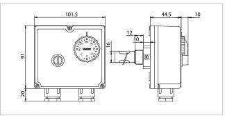
Electrical contact capacity = 10 (2,5) A / 250 Vac Switches = interrupted due to temperature increase or exchange Max. head temperature =  $80^{\circ}$ C Max. bulb temperature =  $125^{\circ}$ C Thermal gradient =  $1^{\circ}$ K/min Protection rating = IP40 Certifications = CE, ENEC03, DIN, PED, EAC
