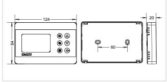
Operating current: 3V DC (2 AAA alkaline batteries) Relay NO Switching current: 2A/30VDC (Resistive load) 2A/250VAC (Resistive load) Temperature measurement accuracy: 0.1°C Operating sensitivity: 0.3°C Operating temperature range: 5°÷30°C Battery life: 1 year (2 x AAA) Operating temperature: -10°÷50°C Storage temperature: -20°÷60°C
