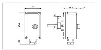
Electrical contact capacity = 10(2,5) A / 250 VacSwitches = interrupted due to temperature increase Thermal gradient =  $1^{\circ}$ K/min Max. head temperature =  $80^{\circ}$ C Max. bulb temperature =  $125^{\circ}$ C Protection rating = IP40 Certifications = CE, ENEC03, DIN, PED, EAC
