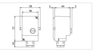
Temperature limiter pre-regulation =  $60^{\circ}$ C Regulation range =  $40^{\circ}$ ÷70°C Tolerance = 0-10K Manual reset Reset temperature = -25K ± 8K range Max. head temperature =  $55^{\circ}$ C Electrical contact capacity = C-1: 0,5 A / 250 Vac C-2: 10(2,5) A / 250 Vac Protection rating = IP40 Certifications = CE, ENEC03, EAC
