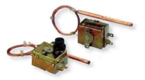
LS1 / LS3 is a capillary thermostat with a liquid expansion probe, unipolar, with safety temperature limiter with manual or automatic reset and with positive safety in case of capillary breakage. It is particularly suitable for boilers, heating systems and in all those appliances where it is necessary not to exceed a maximum set temperature.
