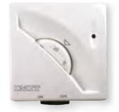
TA3 is a mechanical wall thermostat with saturated steam expansion tank, ideal for regulating home or office temperature. It is available in LED versions, without LED, ON / OFF (to turn off the thermostat without turning the knob), Summer / Winter (to connect and regulate the air conditioning or heating system). This thermostat also offers the possibility to limit or block the set temperature, through the installation of an optional switch under the cover.
