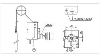
Switches = interrupted due to temperature increase Max. head temperature =  $85^{\circ}$ C Copper bulb =  $125^{\circ}$ C Copper bulb =  $\emptyset$  6,5 x 95 mm Min. capillary curvature radius = 5 mm Certifications = CE, ENEC03, EAC, UL
