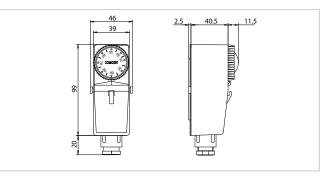
Differential = 8±3K Electrical contact capacity = 16(2,5) A / 250 Vac Thermal gradient = 1°K/min. Max. head temperature = 80°C Protection rating = IP20 Certifications = CE, ENEC03, EAC
