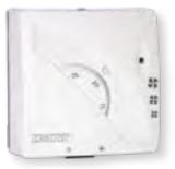
FAN TA3 is an electromechanical steam expansion regulator for fan-coils, radiators and fan convectors. It is ideal for regulating home or office temperature in its two modes of operation: Summer/Winter (to activate the air conditioning or heating functions). It is also equipped with a mechanical three-position switch for regulating fan speeds and to control the hot/cold valve.
