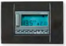
The new FAN / 503S is a DIN 503 built-in fan-coil regulator, with the main functions of the previous FAN 503, for the management and control of 2 solenoid valves (hot and cold) for 2 or 4 pipe systems. The product has been equipped with a new backlit display and a version designed to control the inverter motors, with consequent energy savings.
