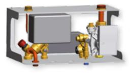
WATERWARM is a compact hydraulic kit, combined with a pellet stove or a thermo-fireplace, which allows the production of domestic hot water and water for heating. It includes a delivery/return group, a brazed exchanger with 20 plates, a diverter valve, a flow switch, an ErP circulator with degasser and built-in drain (only for code 561551) and a pre-wired electrical junction box. Includes white painted cover casing.
