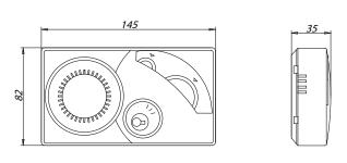
Electrical contact capacity = 5(1) A / 250 Vac Temperature range =  $10^{\circ} \div 30^{\circ}C$ Differential = 0.5 K Insulation class = II Protection rating = IP20 Max. room temperature = 50°C Power supply =  $2 \times 1.5$ V-LR6 AA batteries Operating mode: Manual / Automatic Heating system Form of control: TPI (optional) Certifications = CE, ENEC03
