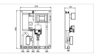
Supply voltage = 230V / 50Hz Max. absorbed power = 100 W Water temperature probe = NTC 1% Operating water temperature = 95°C Max. water probe temperature = 150°C Working room temperature = 0/50°C Storage temperature = 0/60°C Max. fluid pressure = 3 bar Protection rating = IPX40 Certifications = CE
