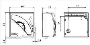
Power supply = 230 Vac Regulation range =  $7^{\circ}$ ÷30°C Differential = 1 K Thermostat contact capacity = 16(2,5) A / 250 Vac Selector switch capacity = 10(2) A / 250 Vac Output = changeover switches Installation = wall Operating mode: Summer/Winter/Anti-freeze System: fan-coil/radiators/fan convectors Certifications = CE, ENEC03, EAC
