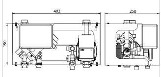
Supply voltage = 230 V / 50 HzMax. absorbed power = 50 WOperating water temperature =  $0/95^{\circ}\text{C}$ Working room temperature =  $0/60^{\circ}\text{C}$ Storage temperature =  $0/60^{\circ}\text{C}$ Max. heating fluid pressure = 3 barMax. fluid pressure ACS = 6 barProtection rating = IPX4D Certifications = CE
