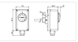
Electrical contact capacity = 10(2,5) A / 250 VacSwitches = interrupted due to temperature increase or exchange Max. head temperature =  $80^{\circ}\text{C}$ Max. bulb temperature =  $125^{\circ}\text{C}$ Thermal gradient =  $1^{\circ}\text{K/min}$ Protection rating = IP40 Certifications = CE, ENEC03, DIN, PED, EAC
