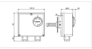
Electrical contact capacity = 10 (2,5) A / 250 VacAdjustable temperature FAN =  $0^{\circ}/60^{\circ}\text{C}$ Internal adjustable temperature LIM =  $30^{\circ}/120^{\circ}\text{C}$ Protection rating = IP40 Max. head temperature =  $80^{\circ}\text{C}$ Max. bulb temperature =  $150^{\circ}\text{C}$ Certifications = CE, ENEC03, EAC
