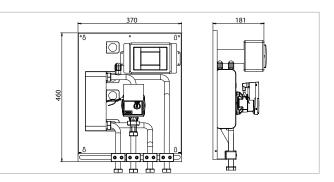
Supply voltage = 230 V / 50 HzMax. absorbed power = 100 WWater temperature probe = NTC 1 % Operating water temperature =  $0/95^{\circ}\text{C}$ Max. water probe temperature =  $150^{\circ}\text{C}$ Working room temperature =  $0/50^{\circ}\text{C}$ Storage temperature =  $0/60^{\circ}\text{C}$ Max. fluid pressure = 3 bar Protection rating = IPX4D Certifications = CE
