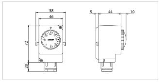
TCR is a liquid expansion boxed thermostat, unipolar, with interrupted or changeover switches, for contact appliances. Particularly suitable for measuring and regulating temperature. Differential = 10±3K Max. head temperature = 55°C Protection rating = IP40 Electrical contact capacity = 10(2,5) A / 250 Vac Protection rating = IP40 Certifications = CE, ENEC03, EAC
