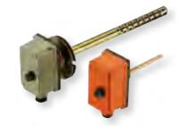
LSC1 is a boxed immersion thermostat, with liquid expansion probe, unipolar, safety temperature limiter with manual reset, fail-safe for capillary breakage, complete with watertight protection pocket. Useful in appliances where safety is required due to the temperature increase.
