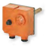
TLSC is a double boxed immersion thermostat, with liquid expansion probes, unipolar, temperature regulator and temperature limiter, fail-safe for capillary breakage, complete with watertight protection pocket. Particularly suitable for appliances where temperature control and safety is required.
