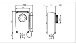
Differential = from 3 to 6°C Electrical contact capacity = 16(2,5) A / 250 Vac Max. operating temperature = 65°C Protection rating = IP54 Certifications = CE, ENEC03, EAC
